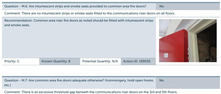
Recommendation: The necessary work should be carried out to ensure the threshold gap beneath the 3rd and 5th floor communications riser doors does not exceed 6mm.
